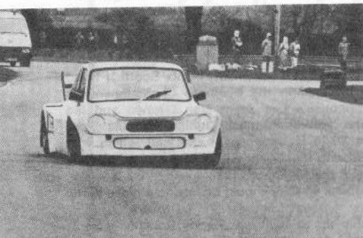
Three seasons ago Laurence Jacobsen ran a particularly fast Imp derivative based on the Chevron B29 chassis. Now Eric Munnoch from Larbert uses the car and has fitted a supercharged 3.5 litre Rover V8 engine. Now that he has the handling sorted out the car is going well.
